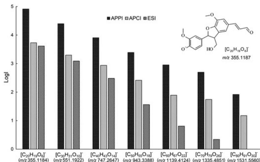
**Figure 3.** Comparison of the peak intensity (LogI) of lignin oligomers in the mass spectra obtained using ESI, APCI, and APPI.
